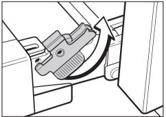
■ Slowly shut the door until the protruding clamps stop the movement. Pull the door upward. See illustration.
